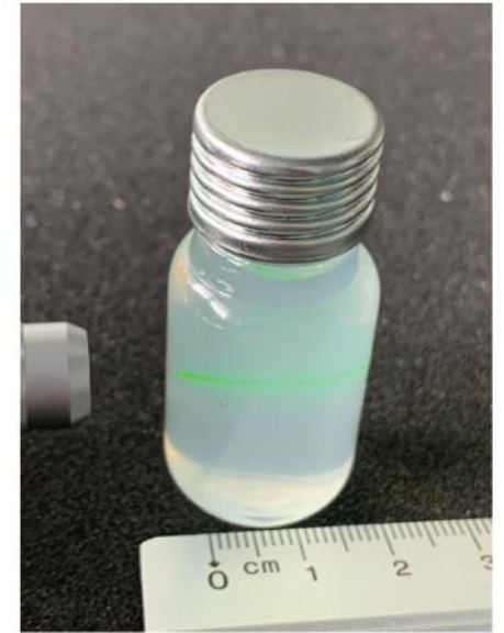
Figure 1. Bottle containing 10 mL of an aqueous dispersion of polypropylene nanoparticles. The dispersion is illuminated with a green laser from the left side to illustrate the light scattering properties.
