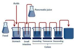
Figure 33: Schematic diagram of the working of a SHIME<sup>®</sup> in vitro cultivation method performed to mimic the in vivo gut construct
