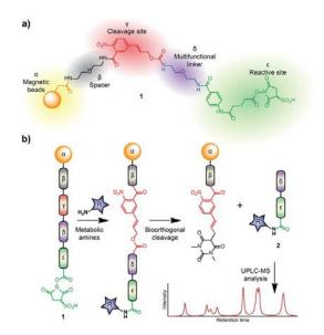
Figure 37: a) Chemical probe design. The reactive site bearing an amine-specific moiety (green) is connected by a multifunctional linker (purple) to the p-nitrocinnamyloxycarbonyl-cleavage site (red). This probe is conjugated to magnetic beads (orange) by a spacer (black). b) The general workflow for analysis of metabolic amines using the chemical probe [41]
