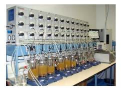
Figure 32: The image shows (SHIME®) system (Simulator of the Human Intestinal Microbial Ecosystem)
