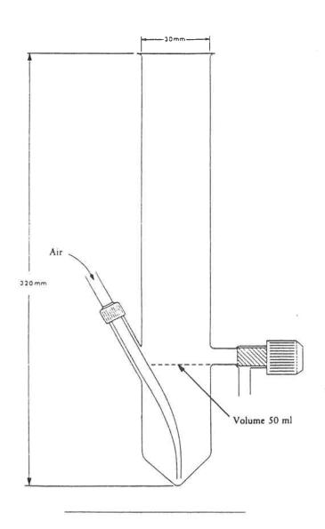
FIGURE A5-3 The Continuous Activated Sludge Apparatus
