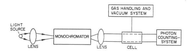
FIG. 1: SCHEMATIC SET-UP OF AN APPARATUS FOR DIRECT PHOTOLYSIS MEASUREMENTS
